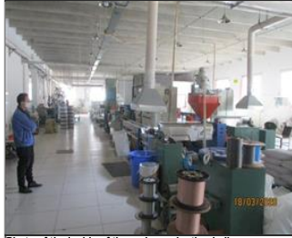
Photo of the inside of the main production hall Extrusion process process.JPG
