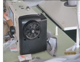
Photo of the inside of the main production hall Belt guard.JPG
